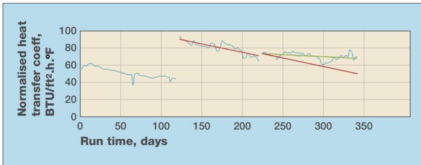
Figure 2 Improved heat transfer on exchanger bundle 2
