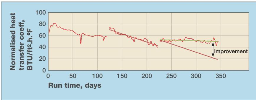
Figure 1 Improved heat transfer on exchanger bundle 1
