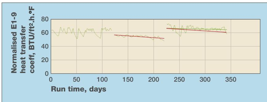
Figure 3 Improved heat transfer on exchanger bundle 4
