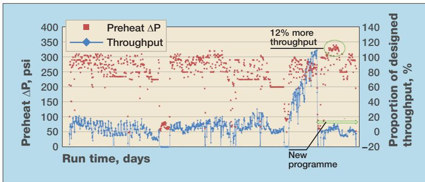
Figure 5 Lower pressure drop and increased throughput
